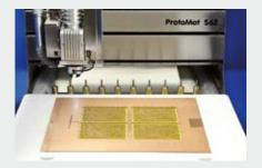
**Integrated vacuum table top** Holds the board material securely in place and maintains perfect flatness.
