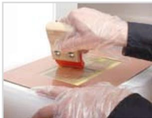
Using the squeegee to apply the conductor
