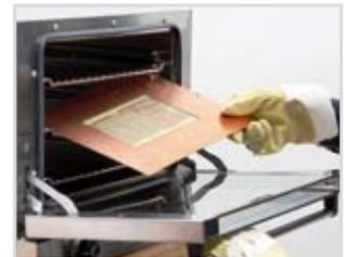
Curing the polymer in a hot-air oven
