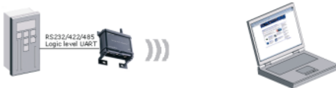
Figure 1. The Serial Port Adapter connected to the controller communicates wirelessly with a Bluetooth enabled Laptop.
