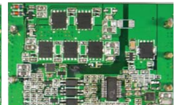
BOTTOM VIEW OF ISL6726EVAL1Z (ACTUAL SIZE: 40x60x16mm)
