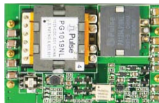
TOP VIEW OF ISL6726EVAL1Z (ACTUAL SIZE: 40x60x16mm)
