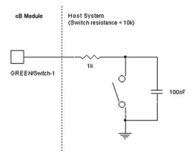
Figure 24: A low resistance restore switch used. Notice the 1kOhm serial resistor.
