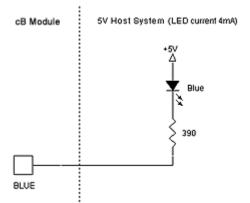
Figure 18: A blue LED can be connected directly to the module if the LED current is below 4mA. A high state (active low) makes the voltage drop over the LED to 2.2V. This is not enough to light the LED.
