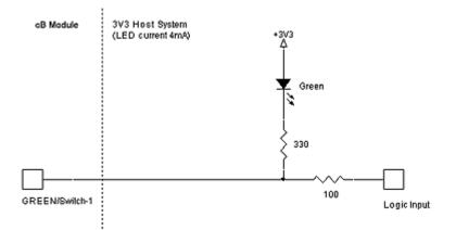
Figure 22: No restore switch used but a green LED in a 3.3V host system. The status of the signal can also be used as input to a host controller.
