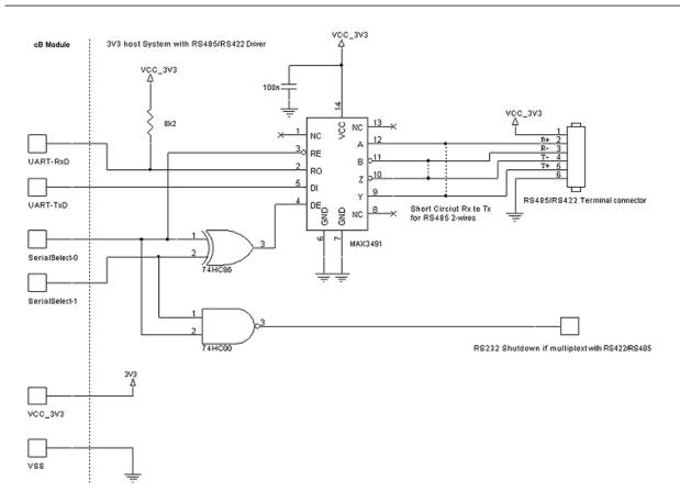
Figure 15: A complete RS422/RS485 transceiver design.
