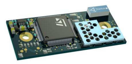
Figure 1: cB-OBS410i-04 OEM Serial Port Adapter with internal antenna
