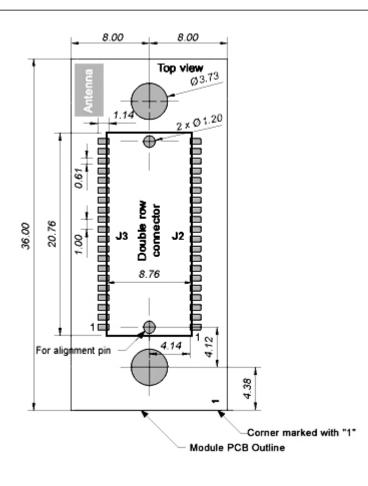
Figure 8: Host PCB layout [mm] for double row connector.
