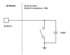
Figure 26: A low resistance function switch used.
