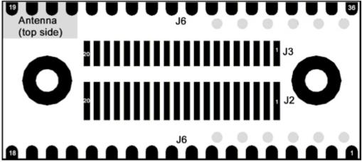
Figure 4: Bottom view of the PCB with the pin numbering of the J2, J3 and the J6 connectors.
