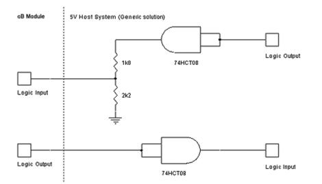
Figure 11: Interface example with logic levels to a 5V system. The gate converting from host 5V output to module input can be repleced with an LVC gate if the voltage divider is removed.
