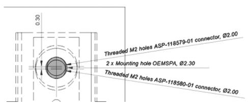
Figure 6: The 2.3mm mounting holes [mm].
