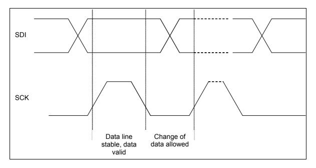
Figure 13: I<sup>2</sup>C, 1 bit transfer
