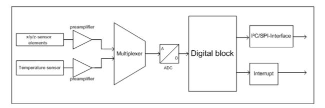
Figure 1: block diagram of BMA180
