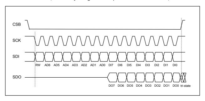
Figure 17: 4-wire SPI sequence
