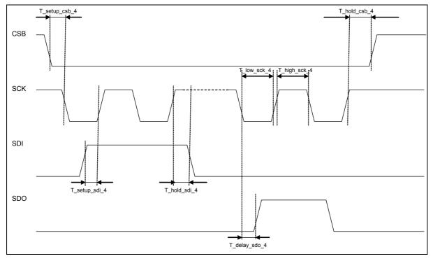
Figure 20: SPI timing
