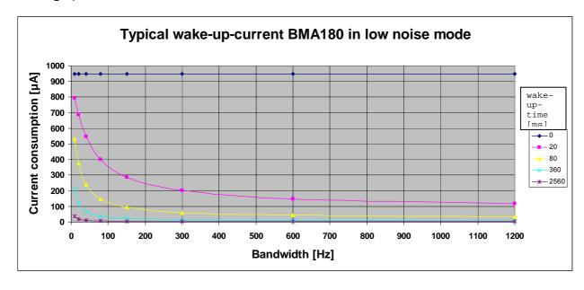
**Figure 3:** Average current consumption in self wake-up mode using high-g or low-g interrupt; here typical values in low-noise mode
