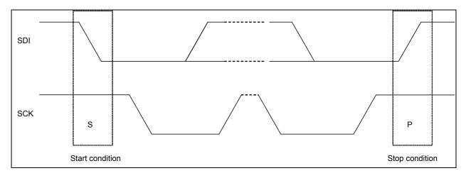
Figure 12: I<sup>2</sup>C start and stop conditions
