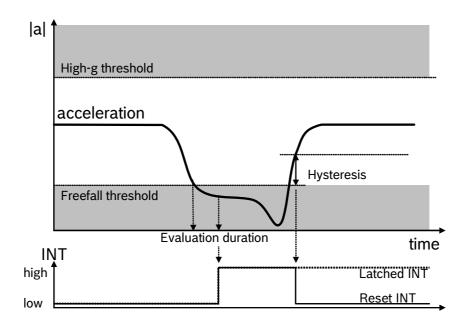
Figure 5: Schematic behaviour in case of low-g detection
