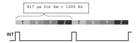
**Figure 4:** Explanation of data ready interrupt: For a bandwidth of e.g. 1.2 kHz the data refresh cycle takes 417 μs to update all data registers. After the final conversion of z-axis the INT pad will be set high. New data can be read out via interface (recommendation: read out within 20 μs after interrupt is high during the conversion of the next temperature value). The interrupt resets automatically after read out.
