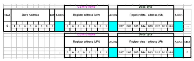
Figure 15: I<sup>2</sup>C multiple write
