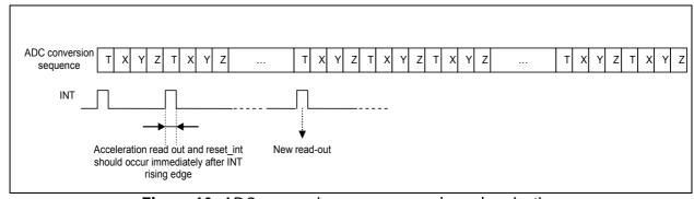
**Figure 10:** ADC conversion sequence and synchronization with read-out of acceleration values
