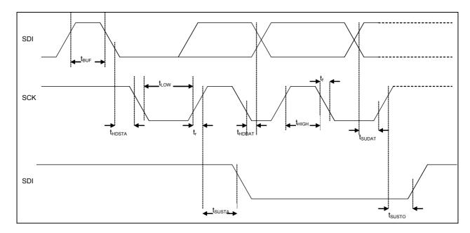
Figure 11: I<sup>2</sup>C timing diagram
