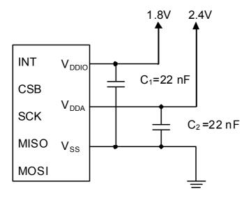
Digital, triaxial acceleration sensor
