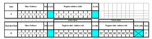
Figure 16: I<sup>2</sup>C multiple read
